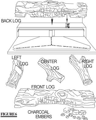
2. Place the back log onto the step located at the back of the combustion chamber. The notch situated at the lower right of the back log should be centered evenly above the pilot assembly.
